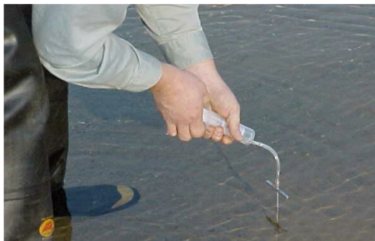
Figure 3: PushPoint Sampling Device a) PushPoint Pore-Water Sampling Apparatus b) PushPoint Sampling Apparatus with Syringe Source: www.mheproducts.com
